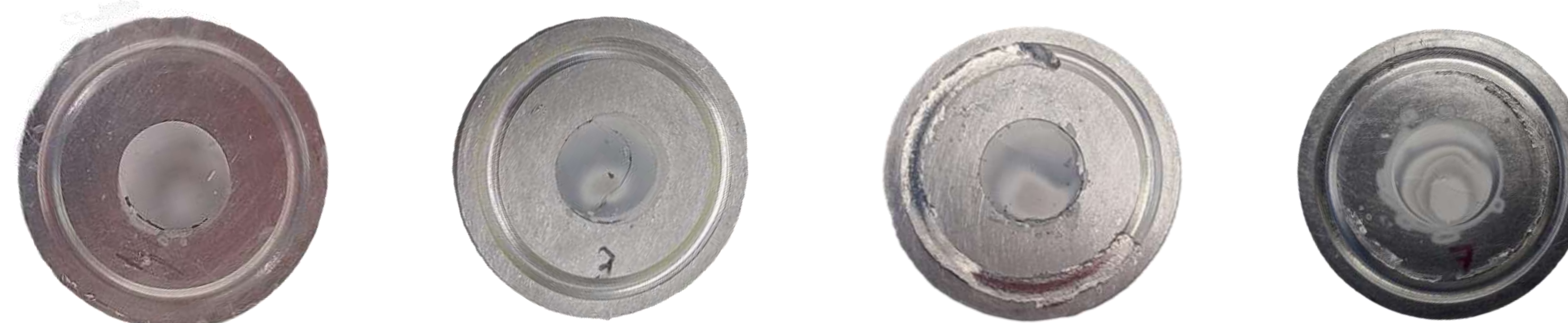
Figure 3: Unsealed Gd 2 O 3 targets post irradiation (from left to right 5 \mu A, 10 \mu A, 15 \mu A, and 20 \mu A)
